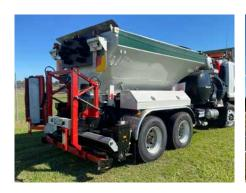
2.4m width of spray sealing, with easily selected control with 300mm segments or narrow strips.
